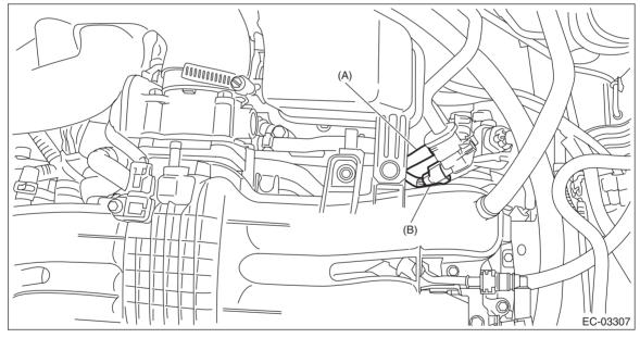
5) Remove the vacuum hose from the purge control solenoid valve.
