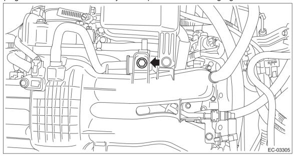
3) Disconnect the vacuum hose from the intake manifold and intake manifold clip (A).
